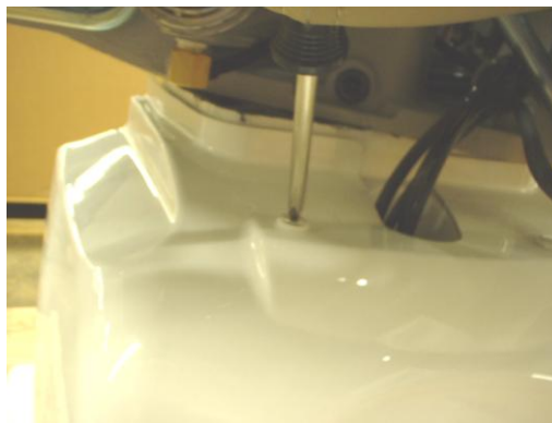
Removing top screw, Dome Casting Cover. (Rear view)
