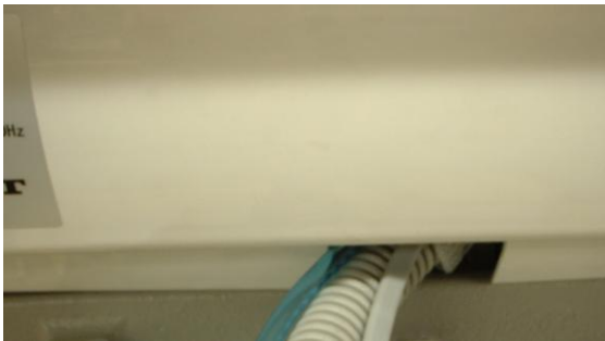
Vac Pac umbilical tubing exits through notched cut-out in front of the seat.
