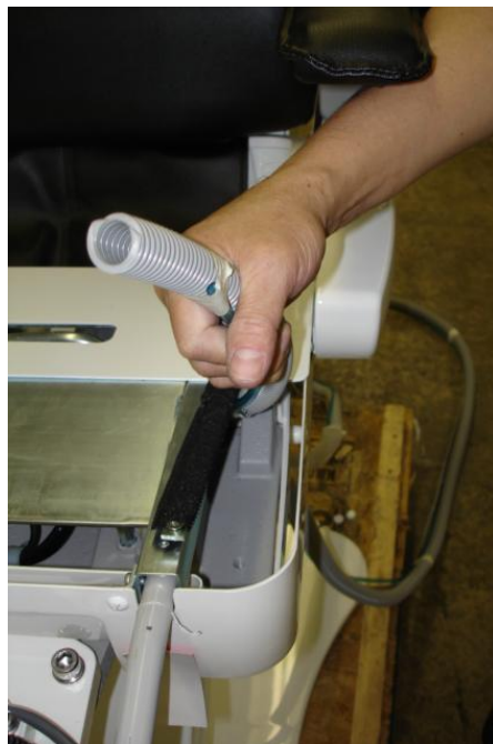
Pull the umbilical upward and route along the outside of the spring area. (View shown-front /right)
