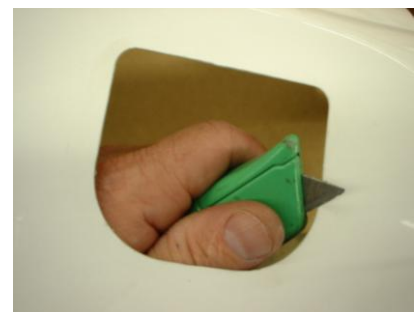
Gradually shave away rough edges around inside of opening
