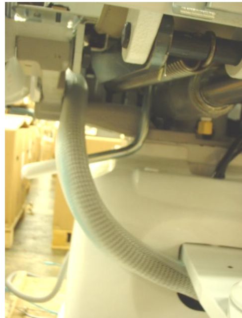
Route the umbilical upward and underneath seat area. (View from rear of chair)
