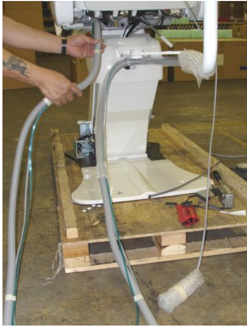
Route the umbilical upward and underneath seat area. (View from rear of chair)
