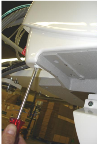
Remove screw underneath the plastic cover in front of the chair (One side only)
