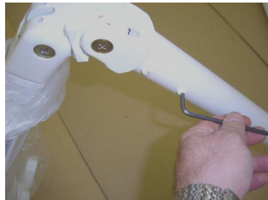
Tighten cap screws to fasten Light Balance arm to Upper Curved
