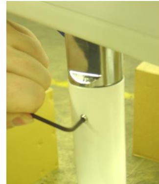
Set Screw and Hex Key Wrench are shipped in a bag attached to the water bottle inside of the J-Box. Insert the 6mm x 5mm set screw into threaded hole on the Swing Arm and tighten to minimize drifting of Balance Arm
