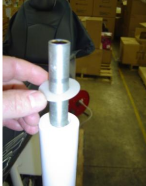
Slip washer onto mounting stud.
