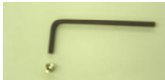
Set Screw and Hex Key Wrench are shipped in a bag attached to the water bottle inside of the J-Box. Insert the 6mm x 5mm set screw into threaded hole on the Swing Arm and tighten to minimize drifting of Balance Arm
