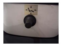
3) Press the "Store" switch located on the right side of the chair base. "Pr" will appear in the display and the chair buzzer will sound. During this time, using the center foot peg on the chair base, push either program 1, 2 or 3 to store the current chair position. (Note: buzzer will sound for 10 seconds then shut off. You must select program 1, 2 or 3 during the sounding of the buzzer)
