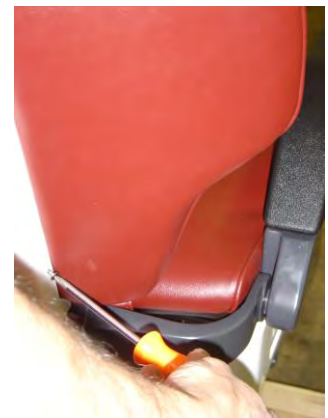
13. Insert machine screws into side holes on the lower portion of the backrest cover and tighten with a Phillips screwdriver
