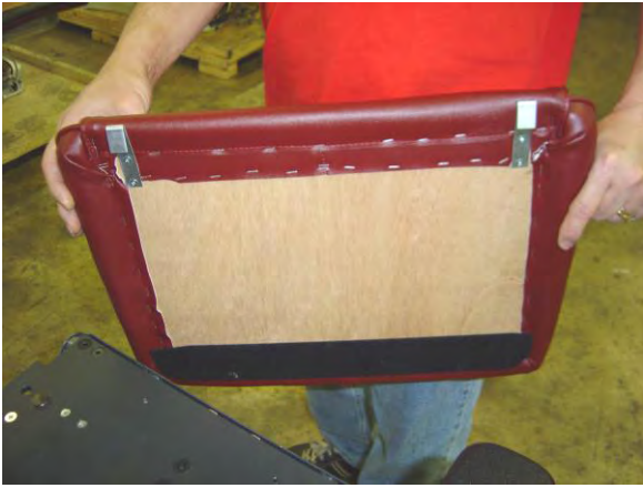
14. Position legrest cushion as shown, with the hooks along the top edge of the cushion, Velcro™ strip at the bottom.
