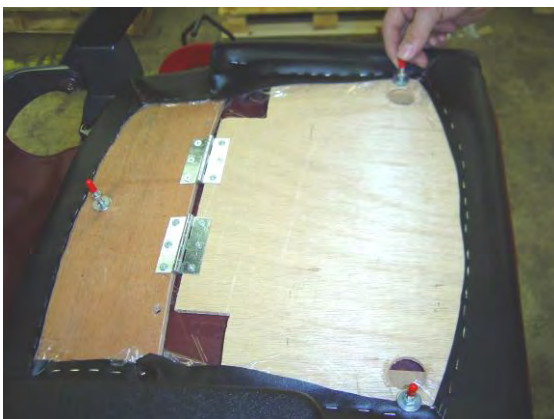
17. Remove red plastic caps from bottom of seat cushion & discard.
