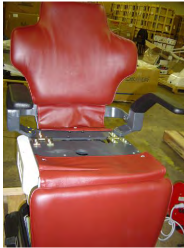
16. Chair with backrest & legrest upholstery attached. Note positioning of backrest and legrest flaps for next steps.
