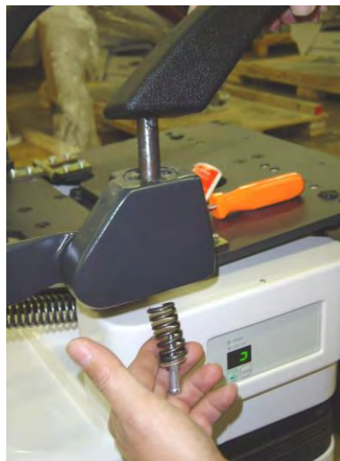
4. Insert armrest into the top of the armrest bracket. Insert washer and spring over screw, then insert into the bottom of the armrest bracket.
