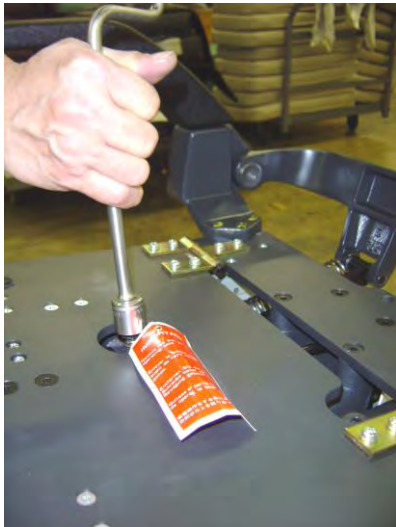
1. Remove tagged red shipping bolt with 11/16" socket wrench.
