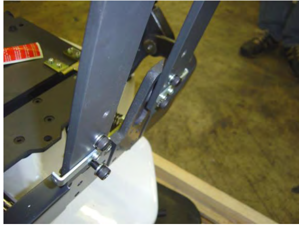
7. Attach backrest support plates to chair using cap screws and split ring washers.
