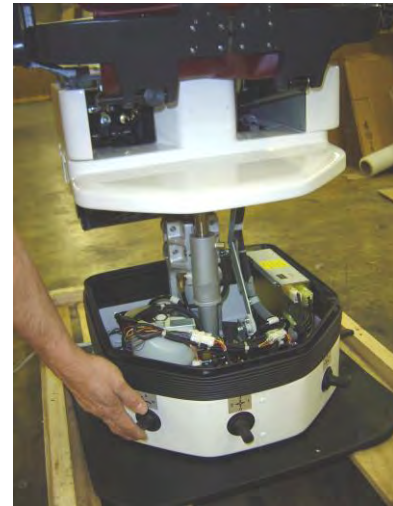
2. Plug chair power cord into an electrical outlet and raise chair base.
