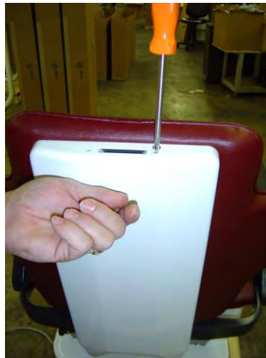
12. Attach plastic backrest cover to chair. Insert wood screws into holes on top of cover and tighten with a Phillips screwdriver.
