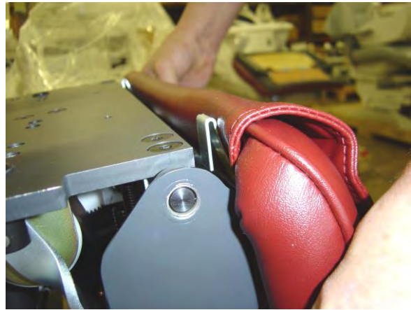
15. Slide cushion downward, hooking legrest cushion on to the legrest frame. Press cushion against frame to engage Velcro™. Note: fold upholstery flap forward while attaching cushion and back over seat plate when procedure has been completed.
