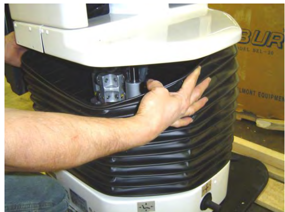
24. Attach the bellows to plastic seat cover. Tuck the upper end of the bellows inside of the lower edge of the cover.
