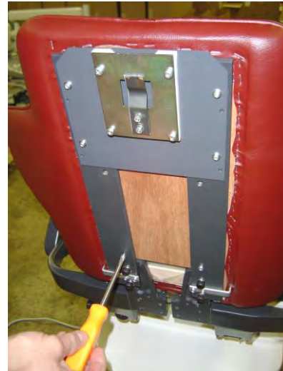
10. Attach backrest to backrest support plates with Phillips head screws.
