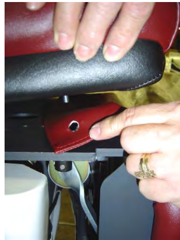
20. Align legrest cushion flap holes with the through holes on the front of the metal seat plate, as shown.
