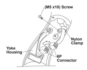
Fig.3-17 Connection 6P Connector in Yoke
