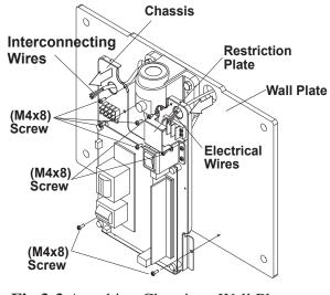
Fig.3-3 Attaching Chassis to Wall Plate
