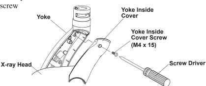
Fig.3-15 Removing Yoke Inside Cover
