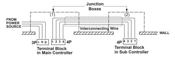
Fig.2-3 Concealed Wiring
