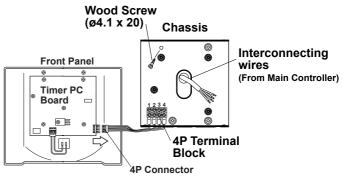
**Fig.3-3;** Attaching Sub Controller Chassis
