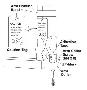
**Fig.3-14** Setting Arm Collar on Balance Arm
