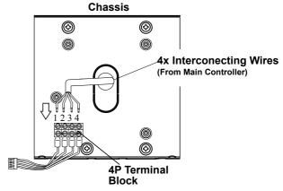
**Fig.3-42** Interconnecting Wires Connection in Sub Controller
