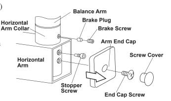
**Fig.3-13** Attaching Balance Arm to Horizontal Arm
