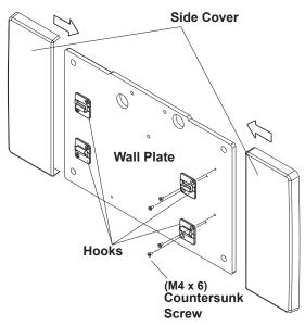
Fig.3-10 Side Cover Installation
