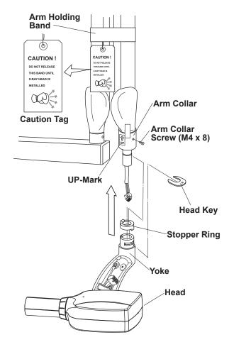
Fig.3-16 X-ray Head Installation
