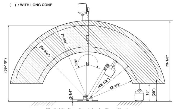
Fig.2-4 Radius of Activity for X-ray Head
