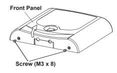
Fig.3-3: Opening Front Panel
