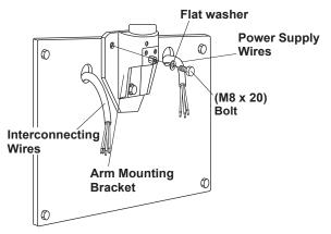
Fig.3-2 Arm Mounting Bracket Installation
