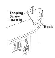
**Fig.3-46** Attaching Hand Exposure Switch Hook
