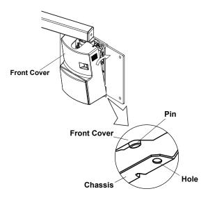
Fig.3-9A Attaching Front Cover-1
