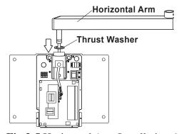
Fig.3-5 Horizontal Arm Installation-1
