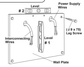
Fig.3-1 Wall Plate Installation
