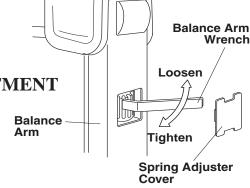
Fig.4-2 Balance Arm Tension Adjustment
