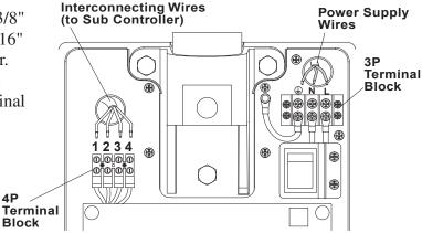
Fig.3-4 Wires Connection in Main Contoller
