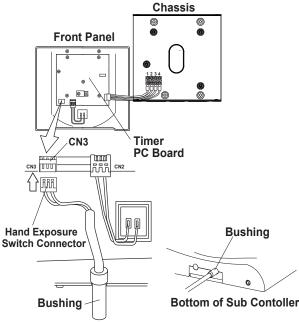
**Fig.3-45** Connecting Hand Exposure Switch
