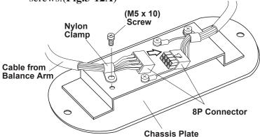
**Fig.3-12B** Connection of Cables and fixing on Bottom Cover
