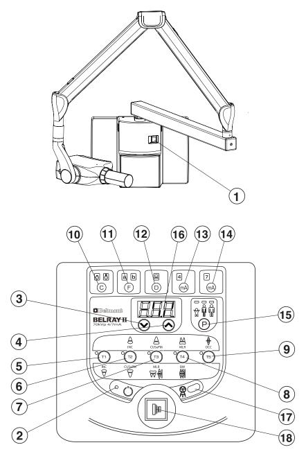
Fig.5-1 Major Components and Control Identification
