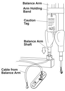
Fig.3-12A Balance Arm Installation
