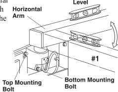
Fig.4-1 Horizontal Arm Adjustment
