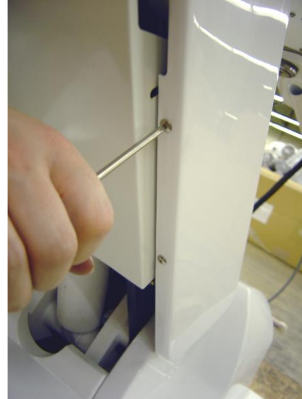
Shown at right, remove 2 phillips screws from the backside of each Link Arm Cover.
