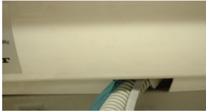
Vac Pac umbilical tubing exits through notched cut-out in front of the seat.
