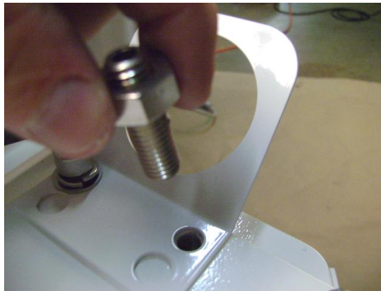
Insert long (35mm) leveling set screw with locking nut through hole in Umbilical Mounting Bracket, as shown above. Nut should be tightened after final leveling of swing arms & unit.
