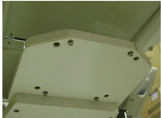
Attached mounting bracket, shown from below. Note (4) 4mm x 10mm Phillips screw heads face down. (These are used for mounting sensor/switch box, if light swing arm is added at a later date)
