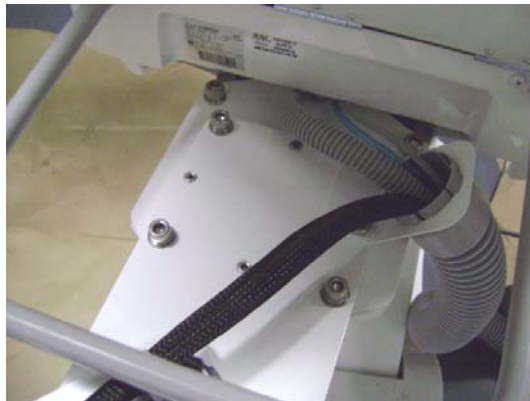
Umbilical from Delivery System is shown installed into Umbilical Duct Hose and routed to J-box. Note: Vac Pac umbilical is also shown routed into Duct Hose in photograph at left.
