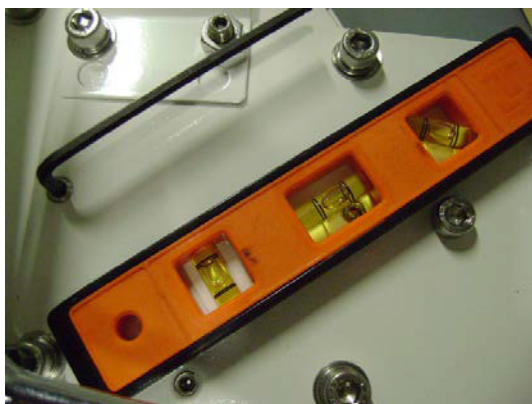
Adjusting (4) set screws for leveling of Swing Arm Assembly
