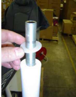
Slip washer onto mounting stud.
