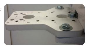
2. Install the Swing Arm Assembly to the top of the adapter plate with the four supplied 3/8-16 x 1.25 flanged bolts. Start two bolts at the back to support the swing arm assembly, then install the (2) remaining bolts.
