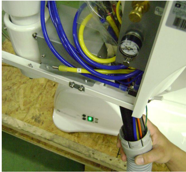
Upper umbilical snaps into the bottom of the PMU frame.
