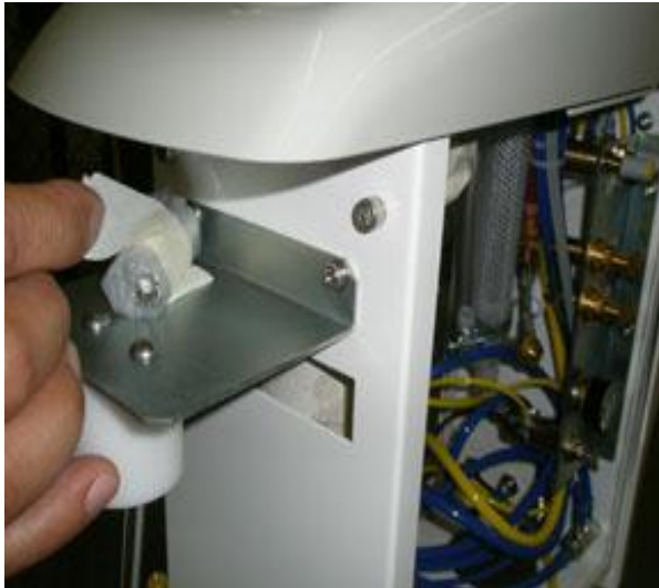
Socket cap screws are taped to the top of the water system bracket prior to shipment from the factory.
