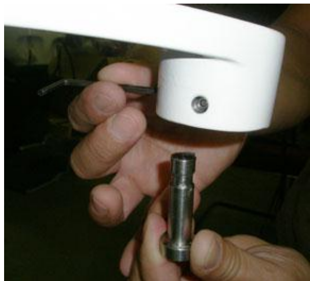
Remove the Pivot Pin by loosening the (2) setscrews with a 3mm key wrench.
