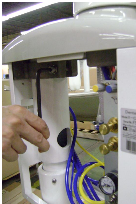
Tightening the PMU mounting clamp to the unit mounting post.
