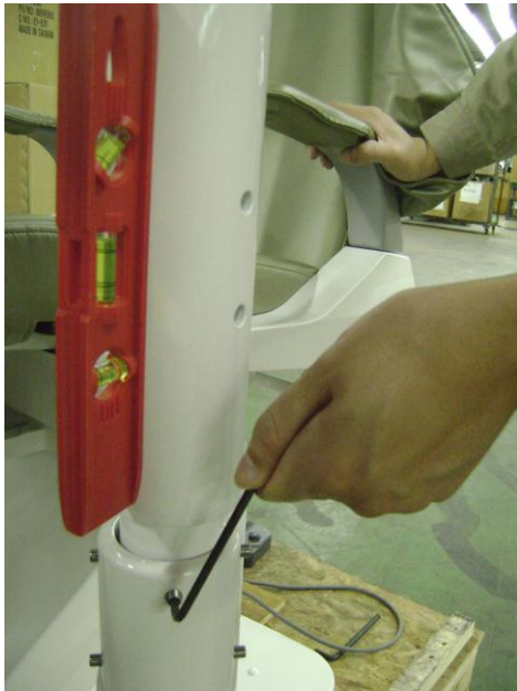
Leveling the unit mounting post with a Bubble Level.
