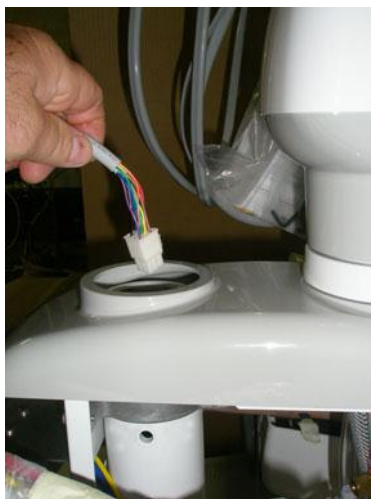
Inserting the upper umbilical from the Dr. Table/ Arm assembly into the top of the unit mounting post.
