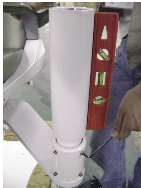
Repeat leveling with Bubble Level placed at 90° to original position, then tighten hub set screws.
