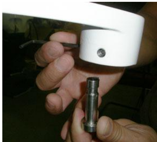
Remove the Pivot Pin by loosening the (2) setscrews with a 3mm hex key wrench.
