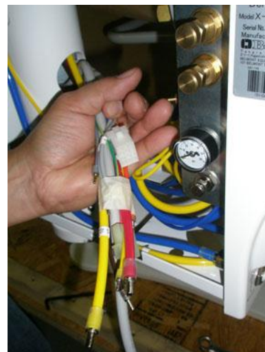
Pulling the upper umbilical tubing into the PMU.
