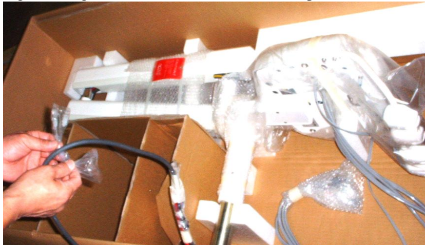
Removing bag of tubing collars from the umbilical prior to insertion into the PMU
