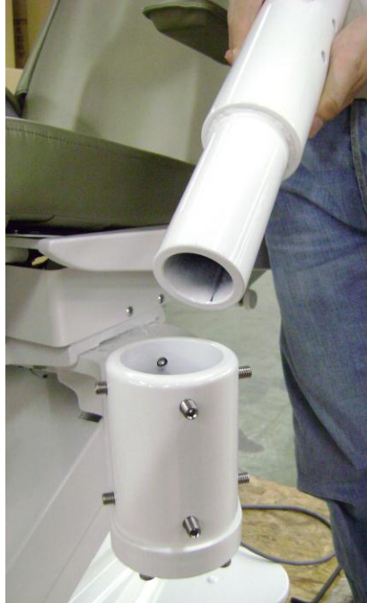
Unit mounting post insertion into the hub of the chair adapter.
