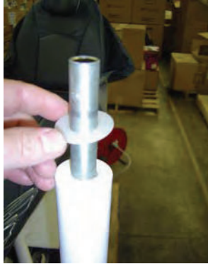
Slip washer onto light swing arm mounting stud.
