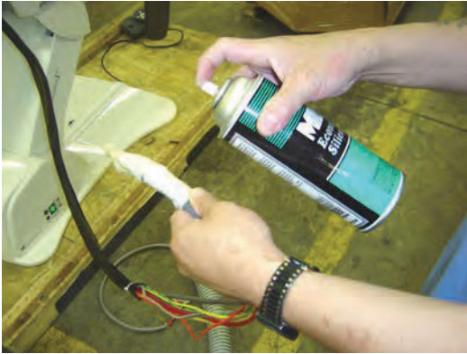
Apply a light coating of silicone spray to the outside of the tubing.
