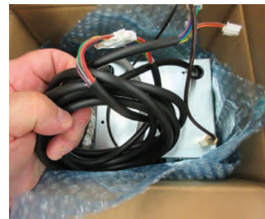
Umbilical wireharness is connected to the Power Supply Box during shipment
