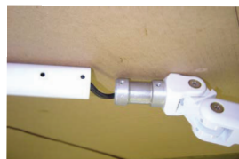
Insert Light Balance Arm Joint into the Upper Curved Post and align holes in post with threaded holes in the Balance Arm Joint for re-attachment with the (2) M6 screws.
