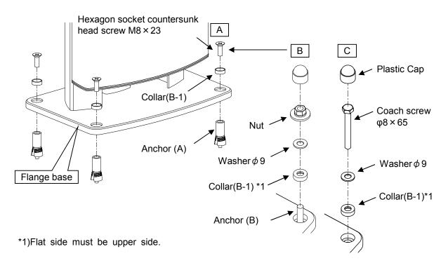
[Construction case, an example of using Anchor (Driving anchor) (A).]
