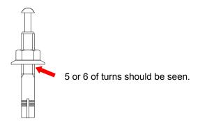
(4). Insert until nut of Anchor (B) has reached the floor.
