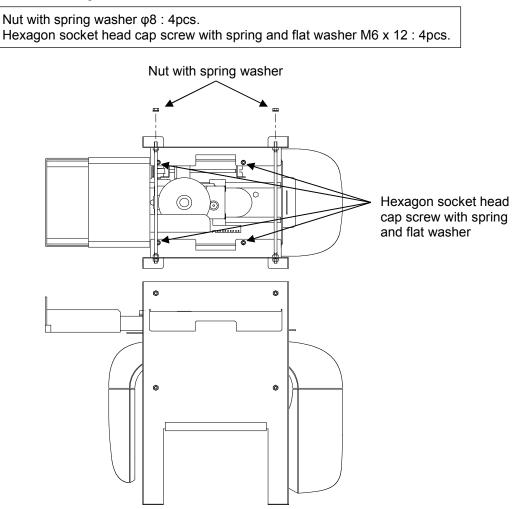
**11.** Remove the protection plate for Median Beam
