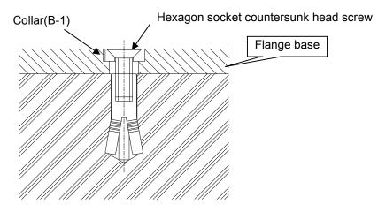
[Construction case, an example of using Anchor (Driving core bar typed) (B).]
