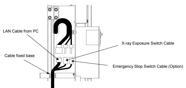
Please make sure to fix a cable to cable fixed base with a cable tie after connecting X-ray Exposure Switch and LAN Cable, so the cable don't come off.
