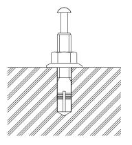
(5). Drive pin in until the edge of it has reached the edge of screw.
