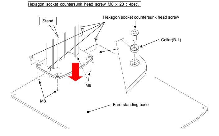
7.2. Move free-standing base to installing position, then fix it at 4 locations with anchor or coac h screw.
