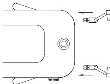
4. 2. By turning Adjuster Knob, open Ear Rods
