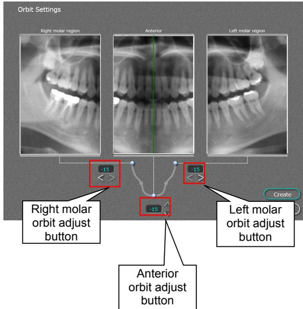
1. By using the Right/Left molar orbit adjust button and anterior orbit adjust button, you can change the slicing orbit plane. Choose the orbit in which the anterior section is clearly shown. Then adjust the molar section so that the size of both left molar and right molar become the same. (Image changes in right/left directions)
