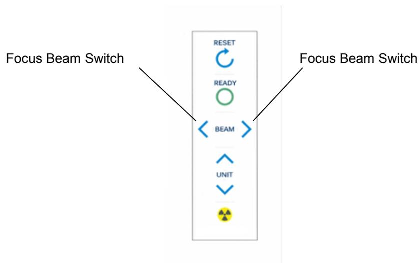
4. 11. Median Beam, Frankfurt Plane Beam & Focus Beam turn on at the same time.
