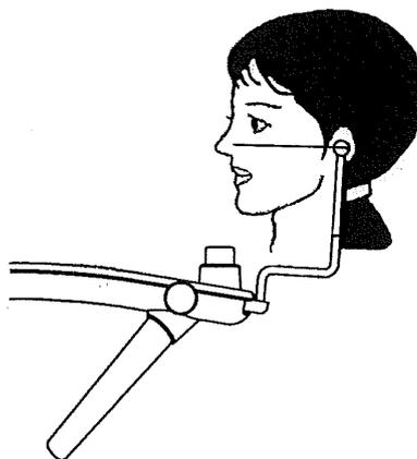
4. 13. Rotate the knob of the Rest Unit ASSY to insert Ear Rod into auricular holes of the patient and lightly fix Ear Rod positions.
