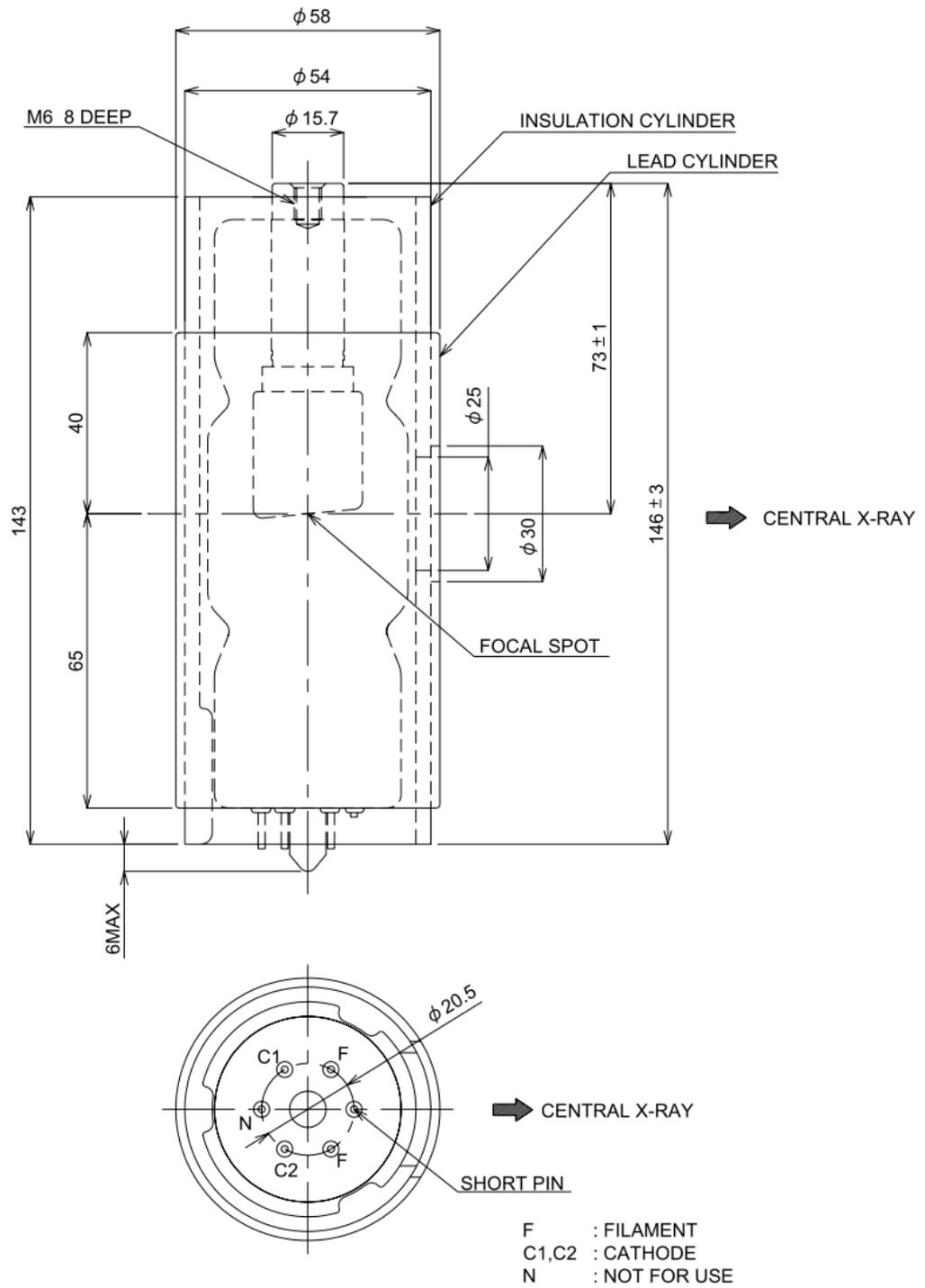
Note: Cathode terminals "C" are connected mutually inside the tube.
