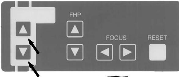
Depress either **UP** **DOWN** key on the Beam Control Panel or the one on the Sliding Unit to move position of Ear Rod(TMJ Frontal).
