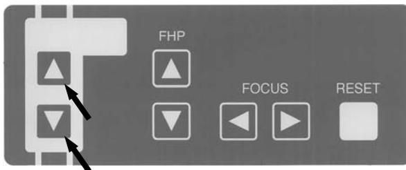
Depress either **UP** **DOWN** key on the Beam Control Panel or the one on the Sliding Unit to move position of Ear Rods(TMJ Lateral). Bring ear rods close to patient's external auditory foramen.
