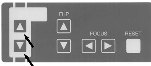
Depress either **UP** **DOWN** key on the Beam Control Panel or the one on the Sliding Unit to move position of Ear Rods(TMJ Lateral). Align ear rods to patient's external auditory foramen.
