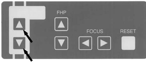
\* Depress either **UP** **DOWN** key on Beam Control Panel or the one on the Sliding Unit to move height of Chinrest (Panorama). Depress up or down key to bring chinrest height close to patient's mandible.
