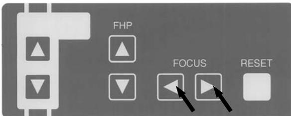
Depress either **Forward Movement** or **Backward Movement** key of FOCUS switch on the Beam Operation Panel to turn Patient Positioning Beams on.
