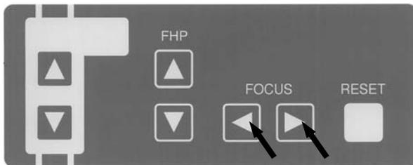
① Depress either **Forward Movement** or **Backward Movement** key of FOCUS switch on the Beam Operation Panel to turn Patient Positioning Beams on.
