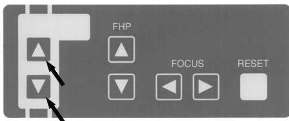
\* Depress either **UP** **DOWN** key on the Beam Control Panel or the one on the Sliding Unit to move height of Chinrest (Maxillary Sinus). Depress up or down key to bring the chinrest height close to patient's mandible.
