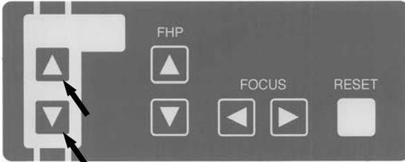
Depress either **UP** **DOWN** key on the Beam Control Panel or the one on the Sliding Unit to move position of Ear Rods (TMJ Lateral).
