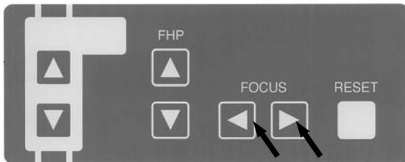
⑥ Depress either **Forward Movement** · or **Backward Movement** key of FOCUS Beam switch on Beam Operation Panel, and align Focus Beam Line with roots of upper and lower anterior teeth.
