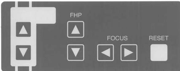
\* Use this to adjust positioning beam lines.
