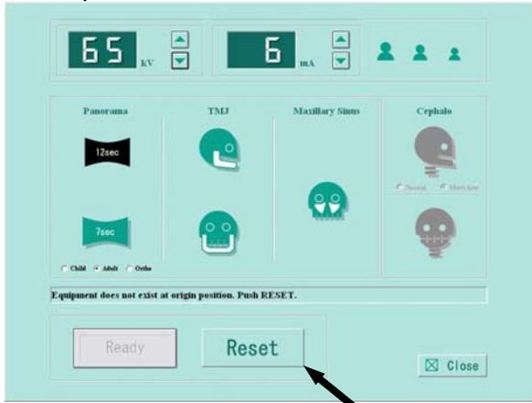
If you receive the message 「Equipment is not at the original position. Push the RESET button.」 Then click the 「RESET button」.
