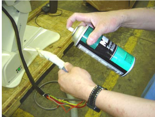
Apply a light coating of silicone spray to outside of the tubing.
