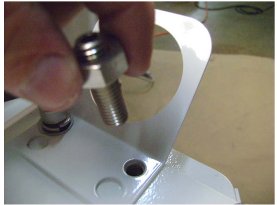
Insert long (35mm) leveling set screw with locking nut through hole in Umbilical Mounting Bracket, as shown above. Nut should be tightened after final leveling of swing arms & unit.
