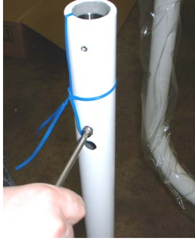
Use Phillips screw driver to remove 6mm x 20mm water bracket mounting screw
