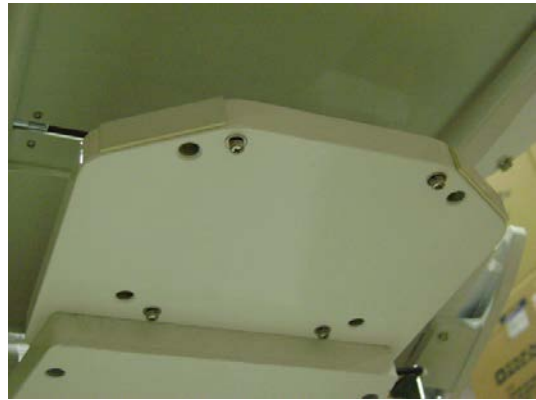
Attached mounting plate, shown from below. Note (4) 4mm x 10mm Phillips screw heads face down. (These are used for mounting sensor/switch box, if light swing arm is added at a later date)
