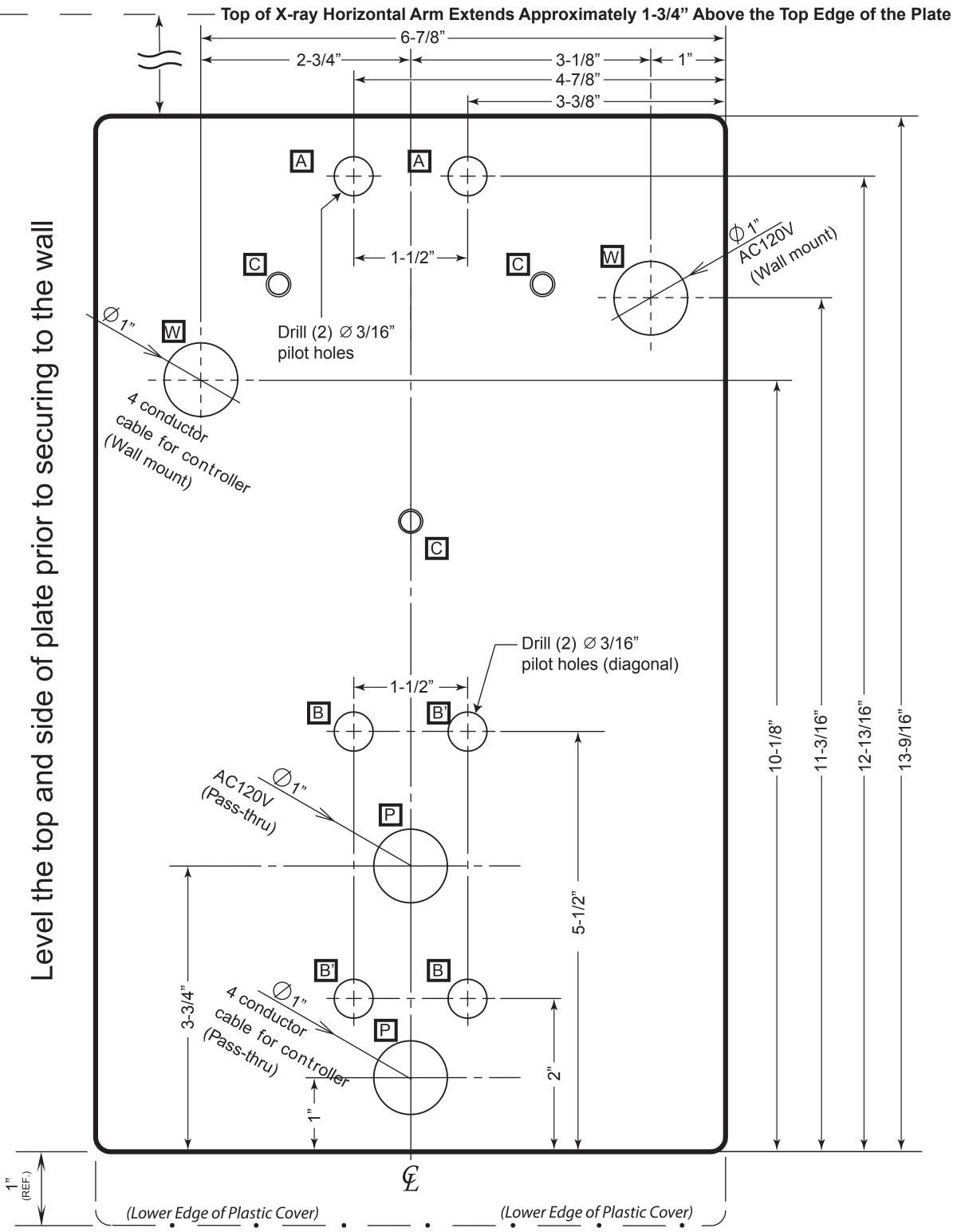
Minimum Mounting Height from Finished Floor to the Bottom Edge of Plate: 34-1/2"
