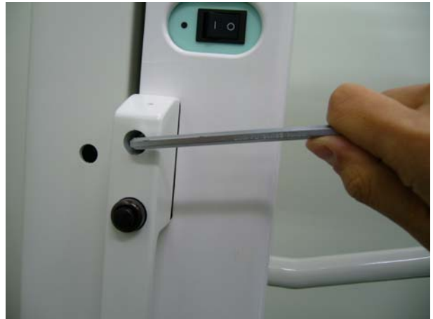
Fix by a cap screw M6×40.
