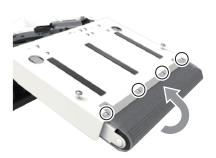
(5) Fix the upholstery with truss head screws, M4  $\times$  6, plated (4 pieces).
