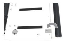
(4) Fold and attach the belt of upholstery with truss head screw, M4  $\times$  6, plated (1 piece).
