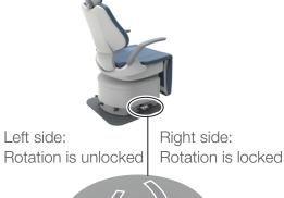
By stepping on the right side of the rotation lock pedal, you can rotate the chair freely.
