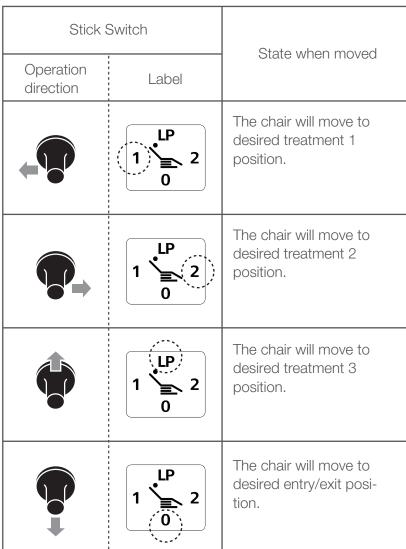
Do not depress the auto operation stick switch for over 5 seconds, because the memorized position in auto mode may be changed. [Reference] Changing Treatment Position and Entry/Exit Position (p. 23)
