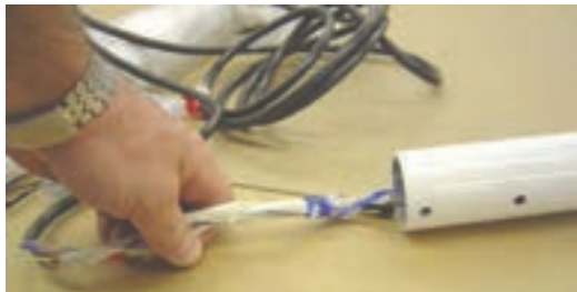
Taped wire harness is wrapped with (blue) flexible ribbon wire and pulled through top end of Upper Curved Light Post. Note: Top of light post has 2 Thru holes as shown above.
