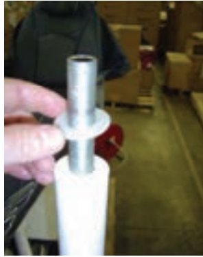
Slip washer onto mounting stud.
