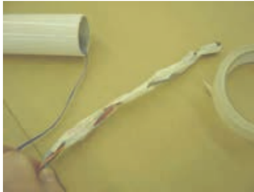
Tape wire harness connectors shown with a single tape wrap in a loose helix.
