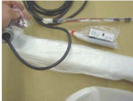
Remove clear plastic tube from connectors, bag with screws and bag with spare bulb and adjustment tool.
