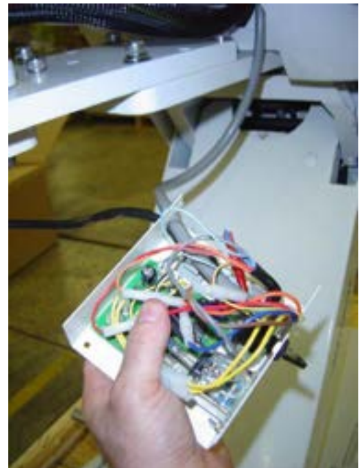
Lower wire harness single pin and double pin connections to the Sensor/Switch Box.
