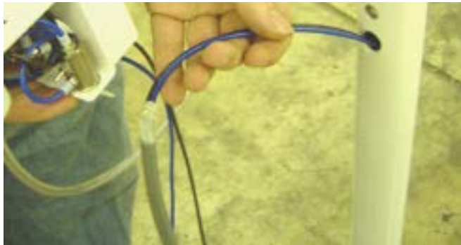
Insert 1/8" blue & brown tubing into the hole on the side of the swing arm and feed tubing down through bottom end of the Swing Arm
