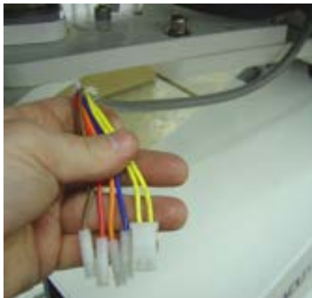
From umbilical wire harness, join brown, red, orange and blue wire with single pin white connectors and yellow wire 2-pin connector to sensor switch box
