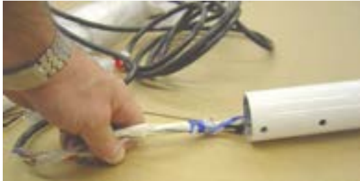
Taped wire harness is wrapped with blue flexible ribbon wire and pulled through top end of Upper Curved Light Post.
