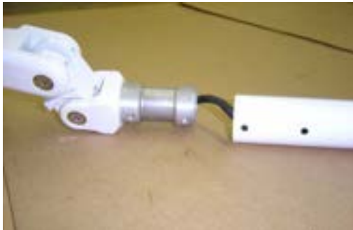
Insert Light Balance Arm into Upper Curved Post. Note: Align through-holes in light post with threaded holes in balance arm prior to insertion.
