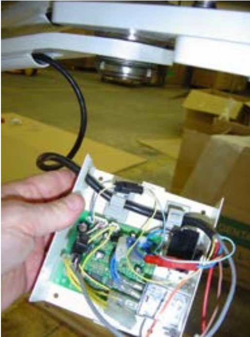
From light wire harness, join 2-pin & 3-pin black sensor wire connectors and blue wire with single pin red connector to sensor switch box.
