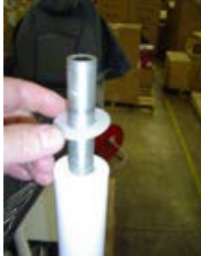
Slip washer onto mounting stud.
