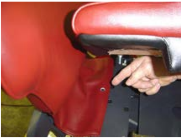
19. Align backrest cushion flap hole with the through hole on the metal seat plate, as shown
