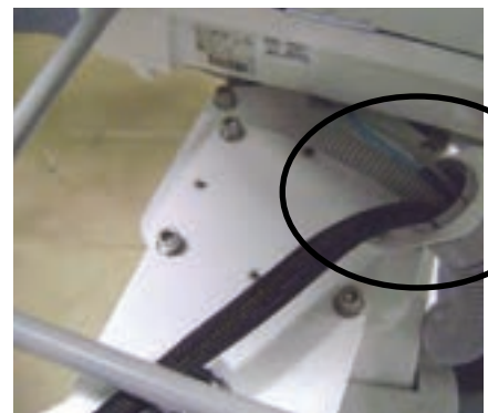
Umbilical Duct Hose is connected to the Umbilical Bracket on the Swing Arm Rotation Plate.
