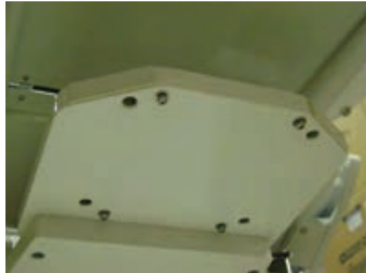
Attached mounting bracket, seen from below. Note (4) 4mm x 10mm Phillips screw heads face down. (These are used for mounting sensor/switch box for dental light )
